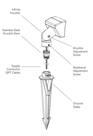
The operating voltage range for this LED luminaire is 9 - 15 volt AC. The Vista electronic driver ensures the LED operates at the intended lumen output while receiving voltage as low as 10.5 volts, and as high as 15 VAC, the U.L. allowed maximum, resulting in a balanced lumen output from the first fixture to the last. Eliminating the dimness issues often attributed to voltage drop.
