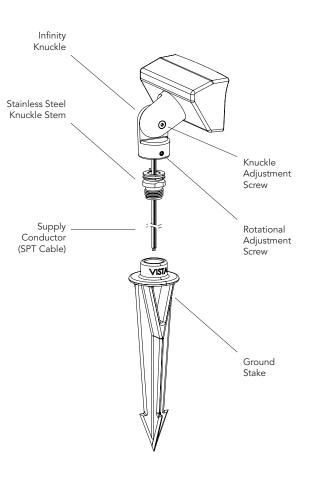
The operating voltage range for this LED luminaire is 9 - 15 volt AC. The Vista electronic driver ensures the LED operates at the intended lumen output while receiving voltage as low as 10.5 volts, and as high as 15 VAC, the U.L. allowed maximum, resulting in a balanced lumen output from the first fixture to the last. Eliminating the dimness issues often attributed to voltage drop.
