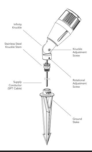
The operating voltage range for this LED luminaire is 9 - 15 volt AC. The Vista electronic driver ensures the LED operates at the intended lumen output while receiving voltage as low as 10.5 volts, and as high as 15 VAC, the U.L. allowed maximum, resulting in a balanced lumen output from the first fixture to the last. Eliminating the dimness issues often attributed to voltage drop.
