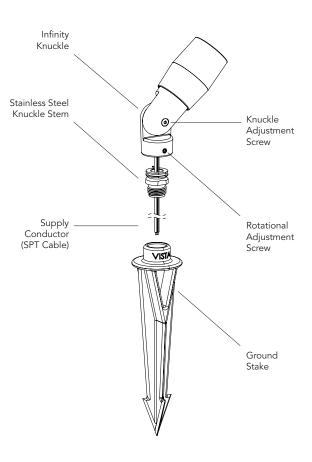
The operating voltage range for this LED luminaire is 9 - 15 volt AC. The Vista electronic driver ensures the LED operates at the intended lumen output while receiving voltage as low as 10.5 volts, and as high as 15 VAC, the U.L. allowed maximum, resulting in a balanced lumen output from the first fixture to the last. Eliminating the dimness issues often attributed to voltage drop.
