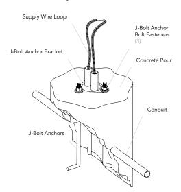
3. Pour the concrete pad to the top surface of the J-bolt anchor assembly bracket. For best results, ensure that the top surface of concrete is smooth and level.
