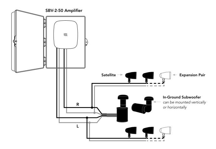
The satellite speakers and subwoofer should be connected in two parallel wire runs and buried in a single trench. The SBV-10-4 system is designed for speakers to be evenly divided between two wire runs with the subwoofer connected to both right and left. Below is a recommended connection.
