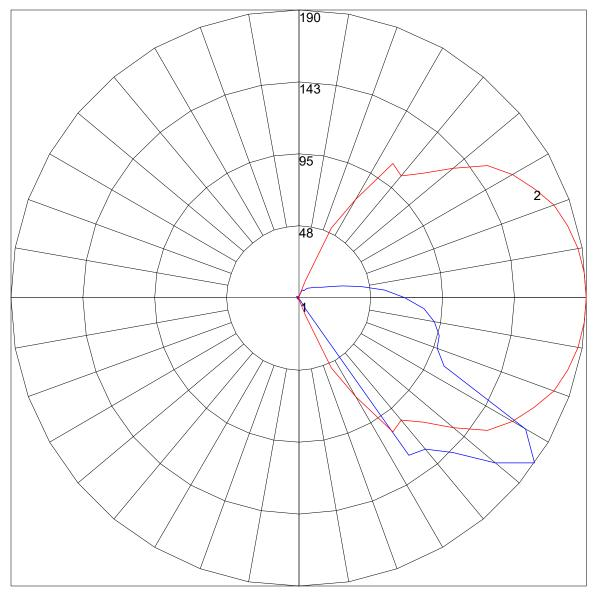
Maximum Candela = 190 Located At Horizontal Angle = 0, Vertical Angle = 55 # 1 - Vertical Plane Through Horizontal Angles (0 - 180) (Through Max. Cd.) # 2 - Horizontal Cone Through Vertical Angle (55) (Through Max. Cd.)
