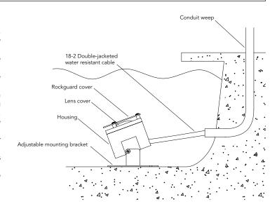
The operating voltage range for this LED luminaire is 6 - 15 volt AC. The Vista electronic driver ensures the LED operates at the intended lumen output while receiving voltage as low as 6 volts, and as high as 15 VAC, resulting in a balanced lumen output from the first fixture to the last. Eliminating the dimness issues often attributed to voltage drop.
