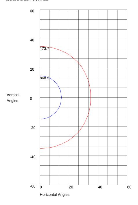
Maximum Candela = 1737 Located At Horizontal Angle = 0, Vertical Angle = 0 50% Maximum Candela = 868.5 10% Maximum Candela = 173.7
