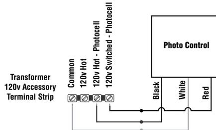
5. Switch power on. The controlled load should turn on regardless of whether you are installing the unit during the day or at night.
