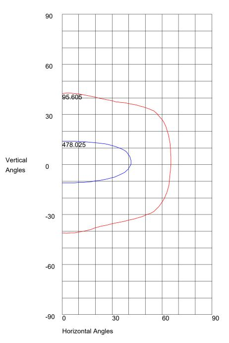
Maximum Candela = 956.05 Located At Horizontal Angle = 0, Vertical Angle = 1 50% Maximum Candela = 478.025 10% Maximum Candela = 95.605
