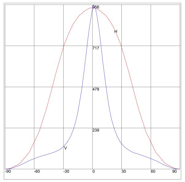
Maximum Candela = 956.05 Located At Horizontal Angle = 0, Vertical Angle = 1
