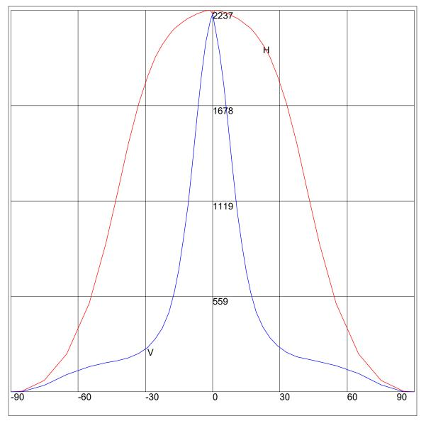
Maximum Candela = 2237.191 Located At Horizontal Angle =-1, Vertical Angle = 0
