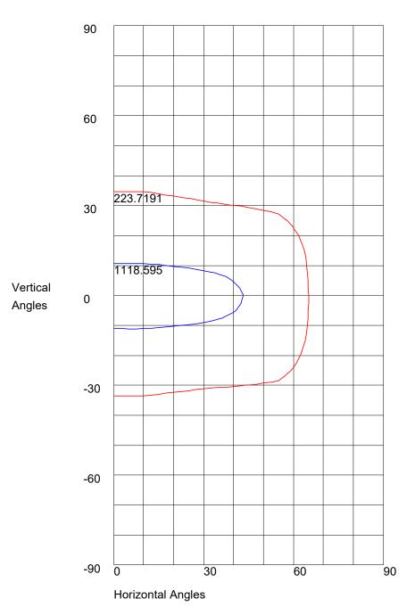
Maximum Candela = 2237.191 Located At Horizontal Angle =-1, Vertical Angle = 0 50% Maximum Candela = 1118.5955 10% Maximum Candela = 223.7191
