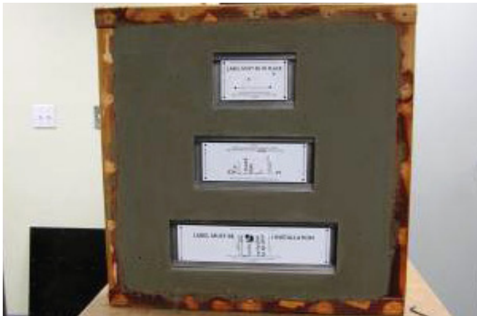
Flush trays shown with pour support plates removed.
