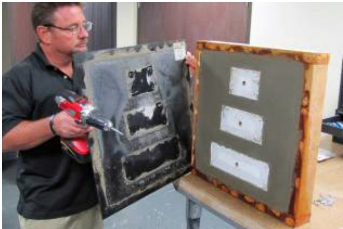
STEP 2 Once concrete is dry, remove form.
