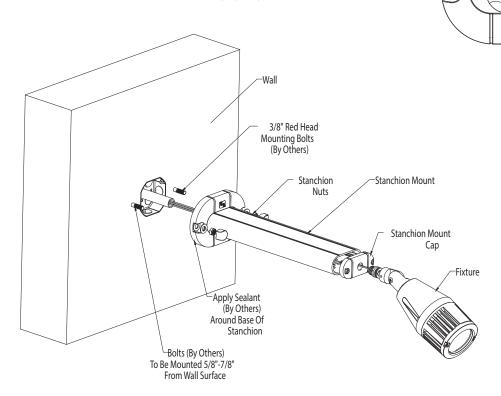
Thru Holes <u>Su</u>itable For 3/8" Bolts (Bolts By Others)
